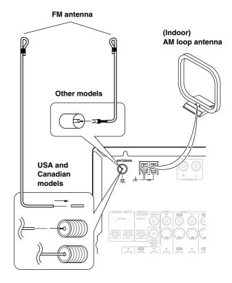
Strip away the insulation from the end of the cable, and fully insert the stripped end of the cable.
